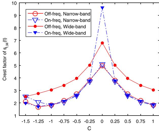
FIG. 7. (Color online) Crest factor as a function of  $C$  for a masker waveform after spectral weighting [i.e., calculated based on  $s_{LM}(t)$ ] using AF parameters estimated for the 60-dB masker SPL in experiment 2. Various conditions for precursors and masker bandwidths are indicated in the inset.
